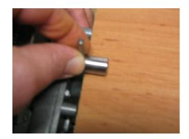
13.Put the motor assembly back. Fasten the 4 screws really tight and check that the motor is in place.
