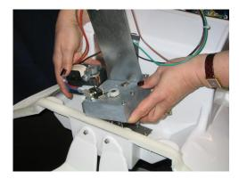
10.Check that the shear pin is off, the axle is smooth and no pin is <sup>►</sup> sticking out.
