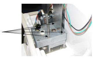
7. Loosen the holder for the cables on the electrical cassette.
