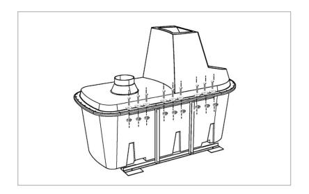
Drill the rest of the holes around the lip of the Kazuba.
