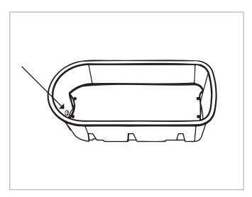
Wipe the rim with the cleaner/acetone before using the silicone for a better join.
