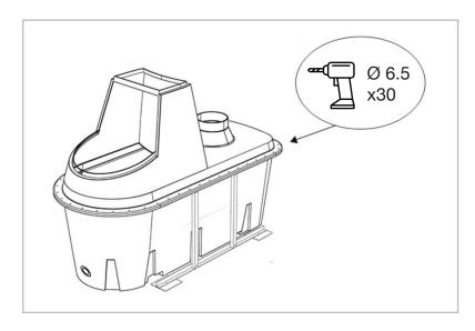
Fit the 50mm bolts supplied into the remaining holes.
